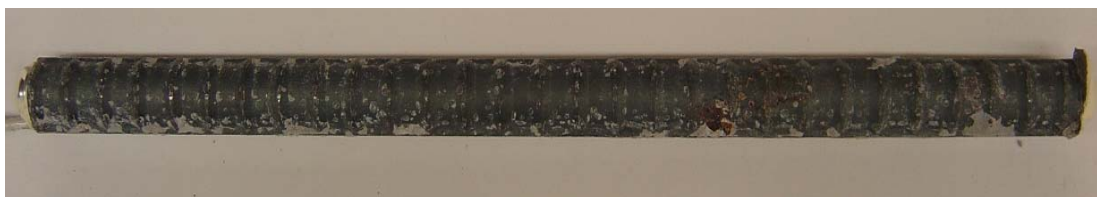
Figure 3.130 – Initiation Beam Test. Conventional steel in the bottom mat (B-N4-Rheocrete-45N-2) showing slight corrosion.
