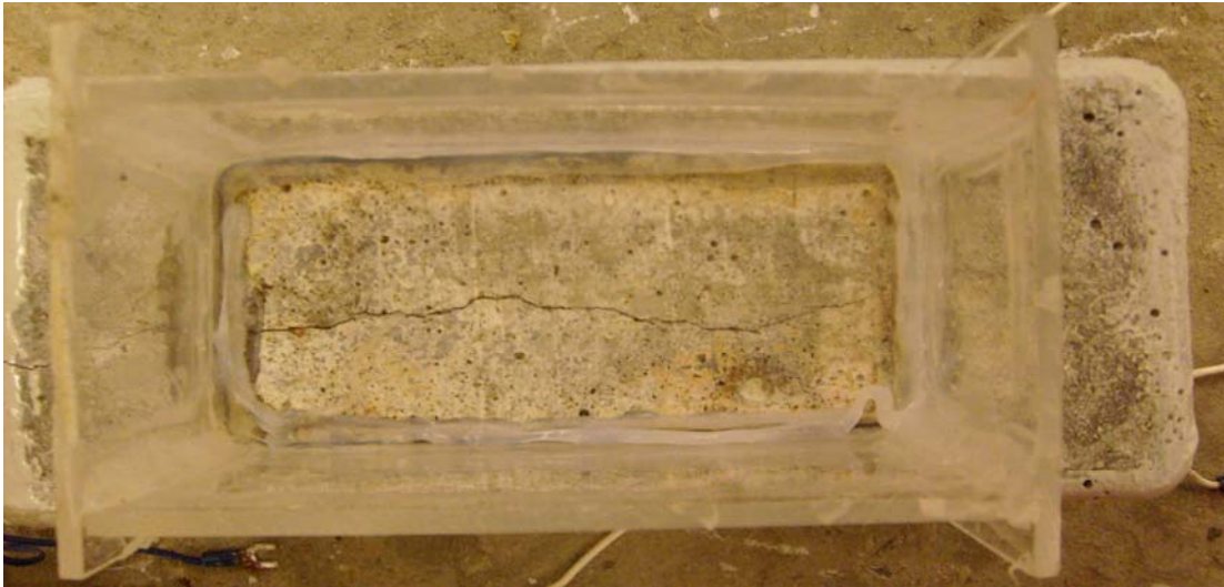
Figure 3.38 – ASTM G109 Test. Specimen with conventional steel (G-N4-Conv.-3) showing a crack on the top surface at week 174.
